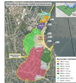
Figure 7: stormwater outfall sub-catchments in the Willard Beach watershed
