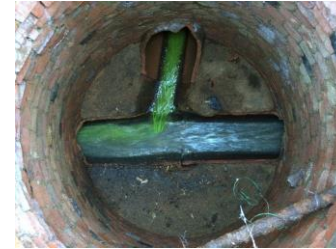
Figure 5: fluorescent dye in drain manhole
